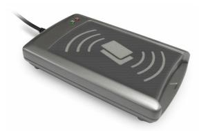
ACR128 is a secure, economically designed dual interface reader that complies to ISO 7816 Part 1-3 Class A and B for the Contact Cards and ISO 14443 Part 1-4 Type A and B for Contactless Cards. This dual interfaces reader offers separated and independent applications for the contact and contactless interface.
